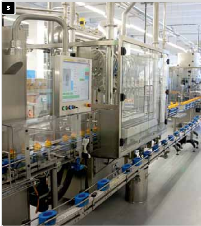
1 Servo controlled piston filling machine for automated filling of thin, thick and foaming fluids from 30–1000ml..
